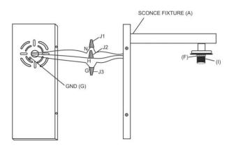
c) Connect the GROUND WIRE of the fixture to the GROUND J-BOX WIRE (usually green or bare). Fasten each together with a wire connector (J) and wrap the connection with electrical tape. Be sure that no wire strands are exposed. If there is no ground wire in the J-Box, use a screwdriver to secure the end of the fixture ground wire to the Ground screw (G) into the back plate (C).
