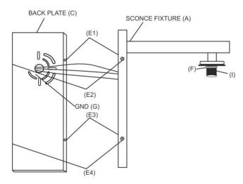
7. Unscrew the shade ring (F) from the socket (I). Fix the Shade (K) onto the socket and tighten the ring clockwise by hand.
